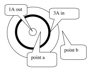
9. (27) A packed bundle of 100 long, straight, insulated wires forms a cylinder of radius R=0.500cm. a) If each wire carries 2A, what are the magnitude and direction of the magnetic force per unit length acting on a wire located 0.200cm from the center of the bundle? (6.34E-3N/m inward.)
