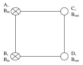
points into the page on the left named A (top) and B (bottom). This is the left side of the square. The right side of the square has the currents come out of the paper with points C on top and D at the bottom. The side length is 0.2m. Calculate the magnitude and direction of the magnetic field at the center of the square.
