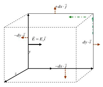
We start by drawing a cube to which we apply Gauss's law. Then we use this law and apply it to the two dimensional projection onto the x-y plane:
