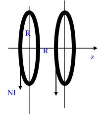
If we put the origin of the z axis into the center of the left coil, the left coil creates a magnetic field at the location z according to formula. The field created by the second coil will be at location z'=z-R. (For z'=0 we are at z=R.) Adding up the fields of the two coils we get: (30.31)
