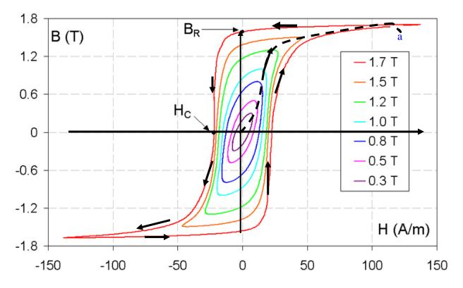
The domains with their magnetic moments inside the iron get lined up to increase the total magnetic field. When the current is turned off, the magnetized domains remain aligned and form a permanent magnet.
