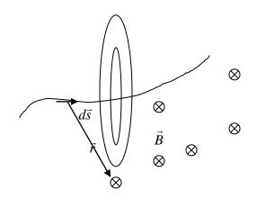
a)Around any current carrying wire curls a magnetic field. The field vectors point into the plane below the wire and come out of the plane above the wire. (Any moving charge has a magnetic field around it.)
