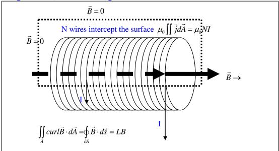
For an idealized situation we ignore the magnetic field outside the solenoid (it is weak), and get for the circulation of B simply BL. If there are N loops, N currents will intercept the rectangular area between the dashed lines; we get
