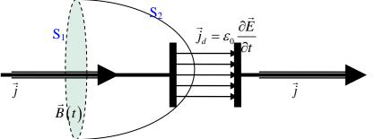
electric field. As we are getting the same magnetic field, we must also get the same "current value" in the empty space between the capacitors.
