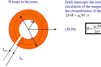
that the Stokes-Ampere surface (a circular sheet of radius R, concentric with the circular magnetic field) intercepts the current N times, whereas the circulation of the magnetic field inside is equal to the circumference of the circle times B:  $2\pi rB = \mu NI \rightarrow$
