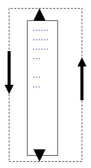
The magnetic field tries to curl around the sheet and cannot do so without intercepting the current, which it cannot do either. The only thing left for it to do is to form a magnetic field parallel to this sheet on both sides of it. We choose as our surface the dashed Ampereian surface which is intercepted by the current. The total current flowing through this conducting sheet is equal to the current density times the cross-sectional area  $A=L\cdot d$ . I = jA = jLd.
