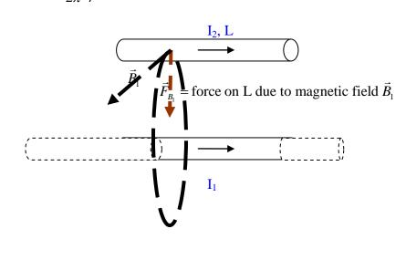
like charges moving in the same direction. They will be repelled if they move in opposite directions. Both wires lie in the same plane of the page, one above the other. The magnetic field of I<sub>1</sub> curls around the wire and points to the outside of the page (towards the viewer) at the wire lying above it. Use your right hand, with the thumb pointing in the direction of current I<sub>1</sub>. The fingers of your right hand point in the
