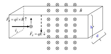
Thus we can measure the drift velocity  $v_d$ . By measuring the Hall potential and the current I we have a way to determine the moving charge density nq. We need to express the drift velocity by the current:
