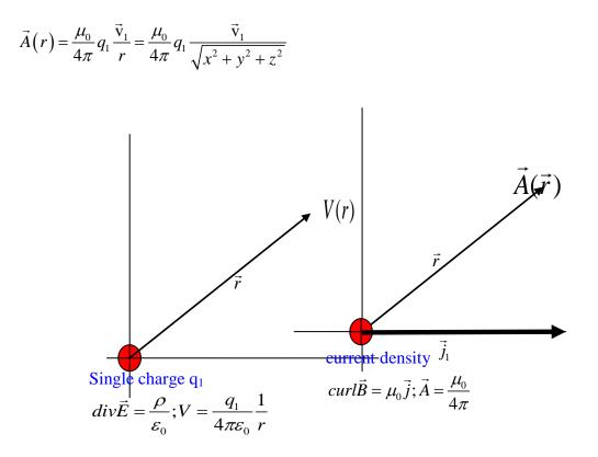
We obtain the magnetic field created by this single moving charge at point 1, by taking the curl of A at point  $\vec{r}$  according to (29.36).
