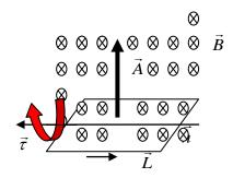
We define the **magnetic dipole moment**  $\vec{\mu}$  as the vector of magitude I (current) times A and in the direction of the surface vector  $\vec{A}$ .
