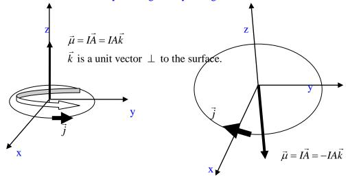
When the magnetic dipole moment is placed into a magnetic field, a torque is being created which re-orients the dipole. The magnetic field will line up the magnetic moment with itself, thus obtaining a position with minimum potential energy for the dipole-magnetic field system. Using the notation of the dipole moment the torque can be conveniently written as:
