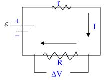
different. We assume a positive current to move from the positive terminal in a clockwise fashion to the negative terminal. We define the emf as follows:
