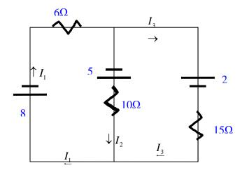
Clockwise:  $-8V - 6I_1 + 5V - 10I_2 = 0$  $-5V - 2V - 15I_3 + 10I_2 = 0$  $I_1 - I_2 - I_3 = 0$  $\begin{pmatrix} -6 & -10 & 0 \\ 0 & 10 & -15 \\ 1 & -1 & -1 \end{pmatrix} \begin{pmatrix} I_1 \\ I_2 \\ I_3 \end{pmatrix} = \begin{pmatrix} 3 \\ 7 \\ 0 \end{pmatrix}$  $A \cdot X = B \Longrightarrow X = A^{-1}B$  $I_1 = -.48A; I_2 = -.010A; I_3 = -.473A$
