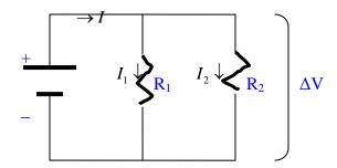
*Conservation of charge or current at a junction point*.  $I = I_1 + I_2$  The potential difference is the same across both resistors.
