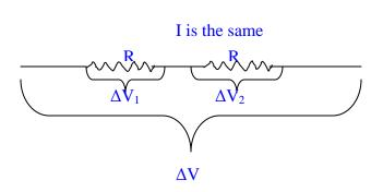
$$\Delta V = \Delta V_1 + \Delta V_2 = R_1 I + R_2 I = (R_1 + R_2) I$$
