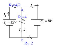
Assign currents through each resistor (current subscript = resistor subscript) in a clockwise direction. For the loop to the left we get:  $12-4I_1-4I_2=0$ For the loop to the right we get:  $-8-2I_3+4I_2=0$ At a junction a we get:  $I_1 - I_2 - I_3 = 0$
